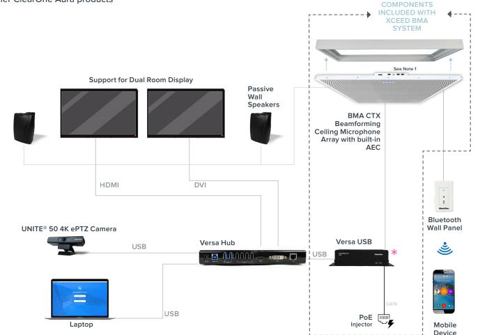
**Note 1:** International Version (Part No. AUR-3200-205-I) P-link input port is shown in drawing above. US Version (Part No. AUR-3200-205-U) P-Link input is accessed through a permanently connected CAT 6 pigtail cable that is terminated with an RJ-45 receptacle.
